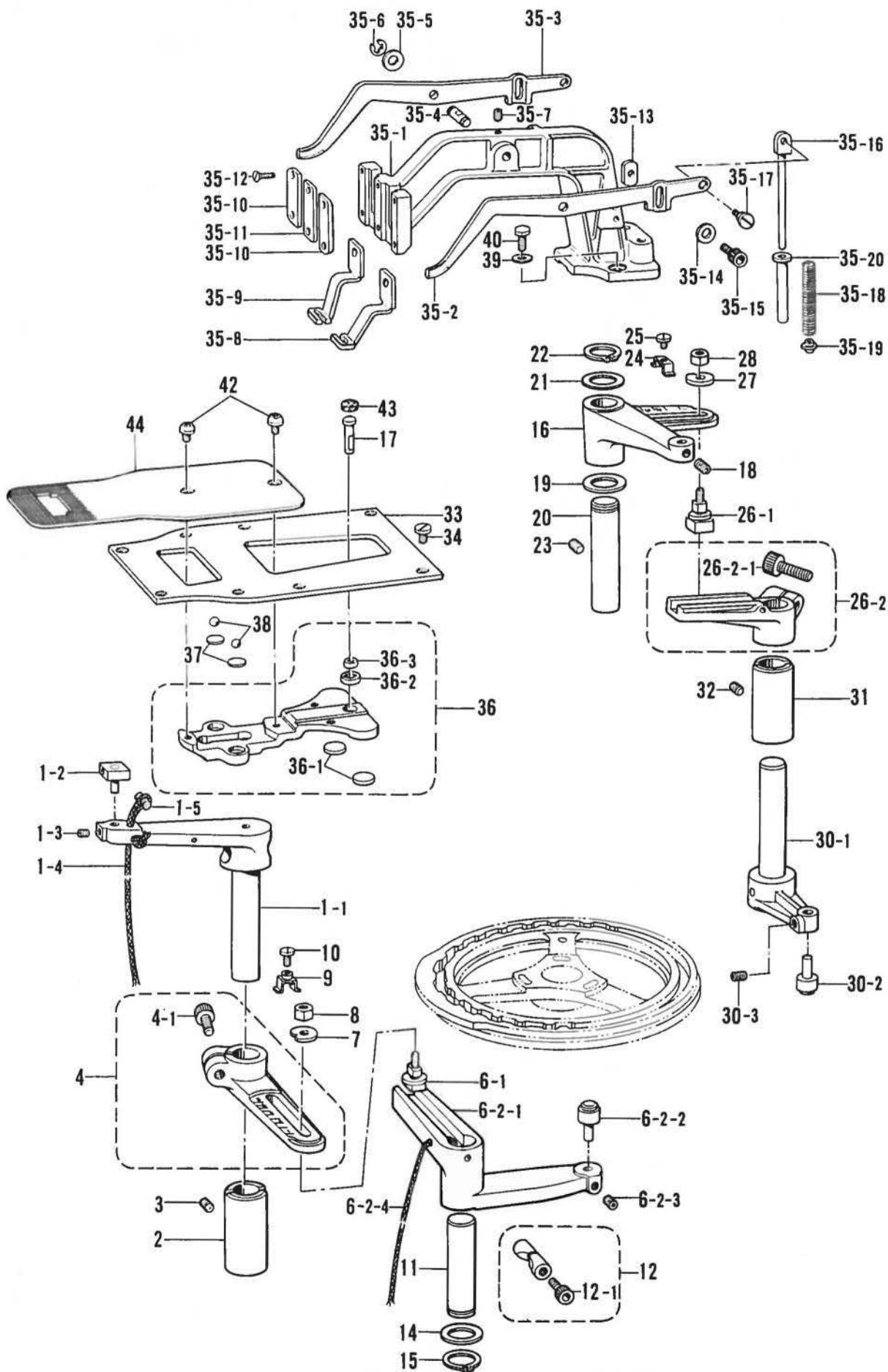
F. 送り関係/Feed mechanism/Transportvorrichtung/
