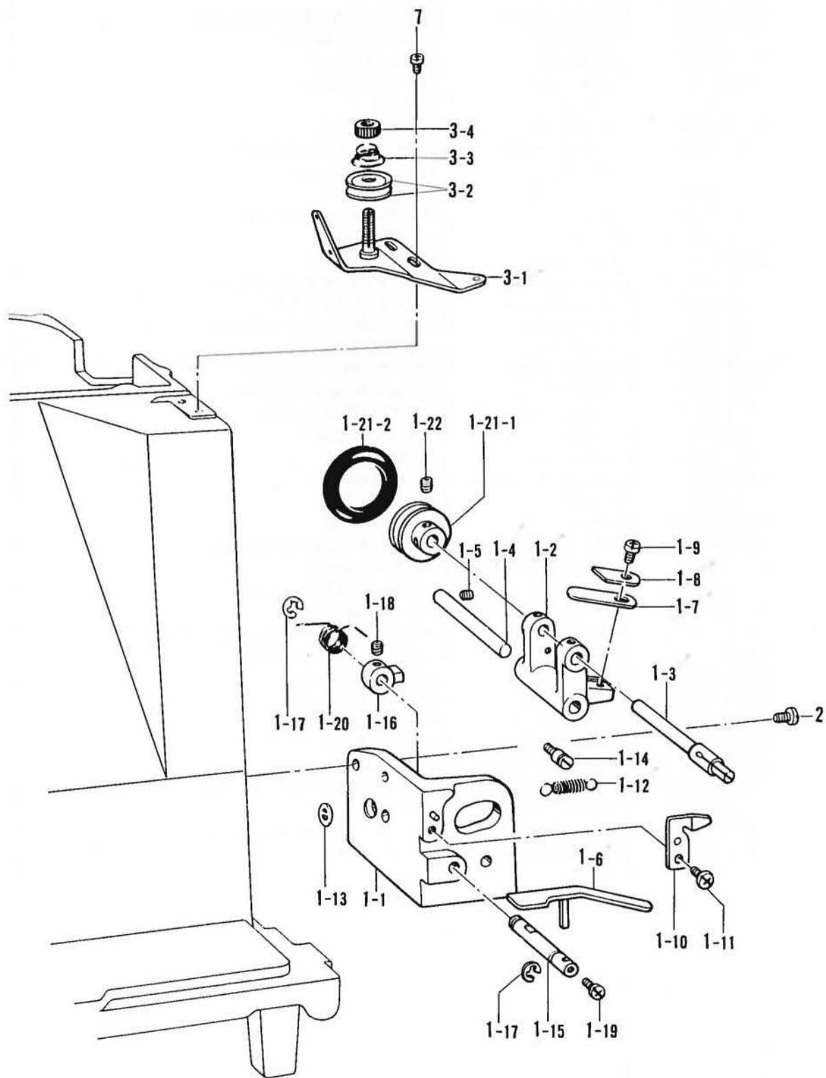
N. 糸巻キ関係 / Bobbin winder mechanism / Spuler /
