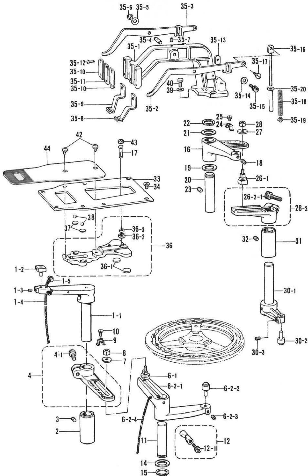
F. 送り関係/Feed mechanism/Transportvorrichtung/
